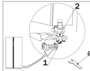
If the doors are uneven and do not close parallel to each other, the refrigerator door must be aligned.
